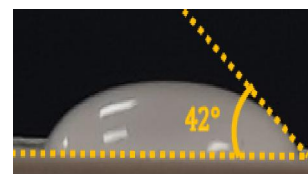
Figure 3. The results of Contact angle of the PU coating
